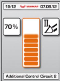
Electrical proportional adjustment of the hydraulic performance of the 3<sup>rd</sup> and 4<sup>th</sup> circuits.
