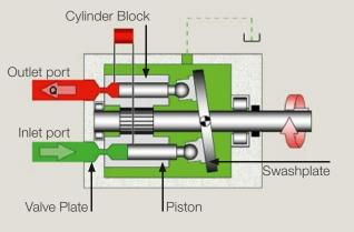
Unlike industry standards for this category of machines, Yanmar is using variable axial piston pump which adapt the flow and the pressure to the load, allowing smoother operation and improving the comfort of the operator. The pump flow of 2 x 11 l/mn and its high working pressure (210 bar) also enable to improve the productivity of the machine and its speed in working motion.
