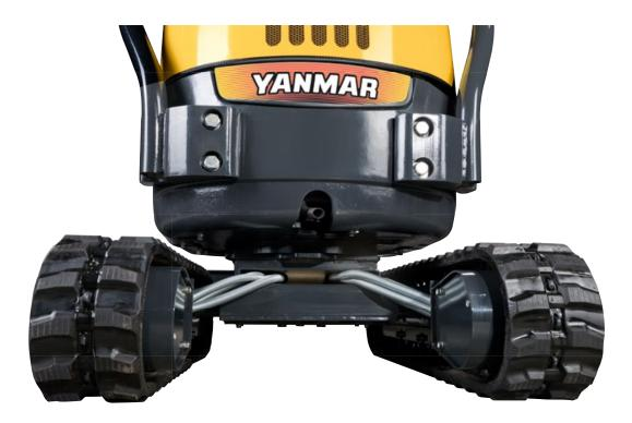
The ViO12 has an operating weight of 1235 kg and the longest undercarriage of its class with 1440 mm. This results in a real improvement of the operator's comfort. He benefits from a smoother drive and increases his productivity.
